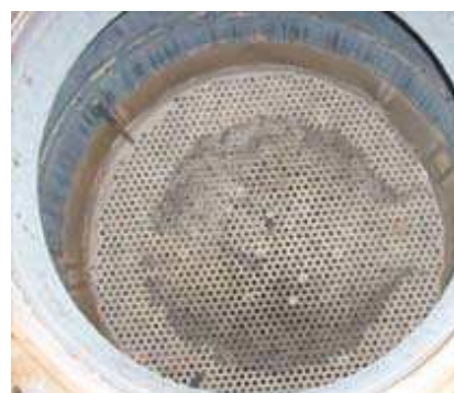
a) Ring liquid divider of NIIK design – deposits are located on the same distance from the wall
