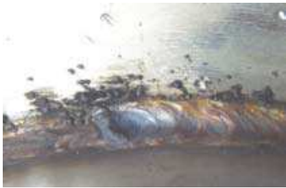
d) lack of shielding gas during welding – gray color of the joint
