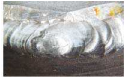
e) cracks nozzle welding joint
