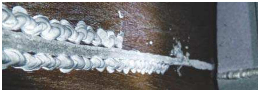
b) welding joint geometry deviations – welding at low amperage
